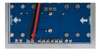
Then, solder then to the LED (the red wire is connected to the longer pin).
