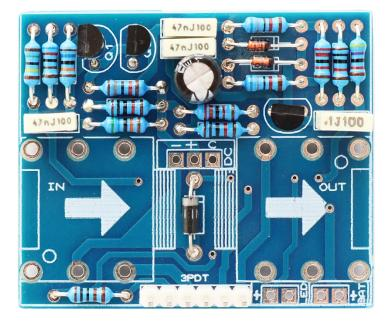
Solder the capacitors and transistors. If you have troubles reading the values, check out our <u>"Reading Part Values"</u> tutorial. Pay attention to the orientation, as well as to the polarity for electrolytic capacitors.
