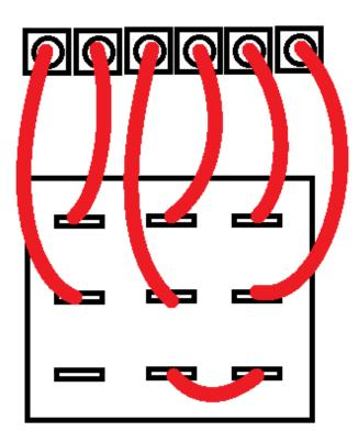
If you prefer to solder the 3PDT directly to the board, you can wire it as shown in the schematic. We recommend to use the **provided 3PDT PCB adapter** to make the soldering easier.
